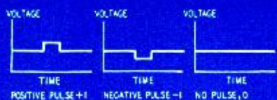
Fig. 1—Pulses are used in electronic computers to represent information. A positive pulse may mean +1, a negative pulse -1, and no pulse 0. Other pulse combinations are sometimes also used.
