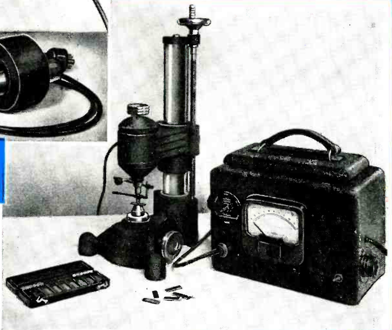
Photo B—The combined inductance-capacitance instrument in a setup to show the stress-strain relation of a steel sample.
